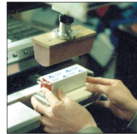
USA Trains uses a pad press to transfer ink onto the railroad car. They have a reputation of having the best printing in the business.
